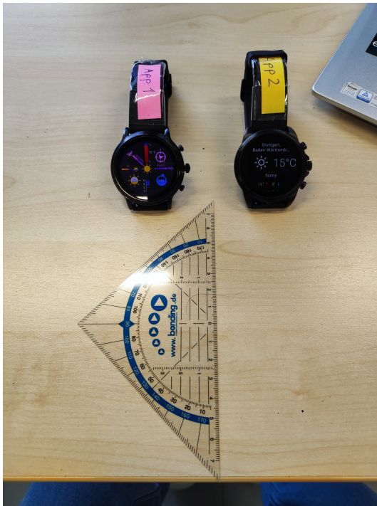
(a) The two watches were placed at a distance of 15 cm from the table border, and with a distance of 2 cm from each other.
