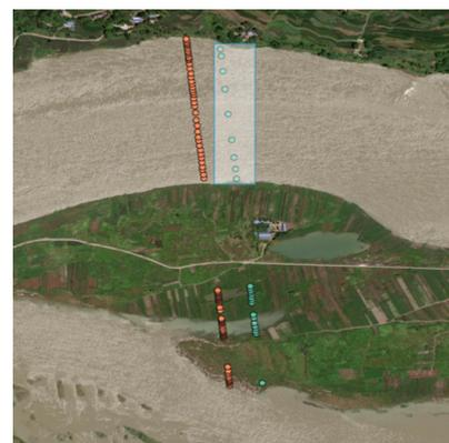
From figures above the orthometric heights from strong and weak beams can be derived separately. For each beam the data file of the elevation would be downloaded and repeat the previously mentioned steps to calculate the water level.
