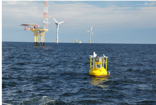
Figure 2.5: Fraunhofer Wind Lidar Buoy during a trial next to the FINO1 met mast within the German bight [3].
