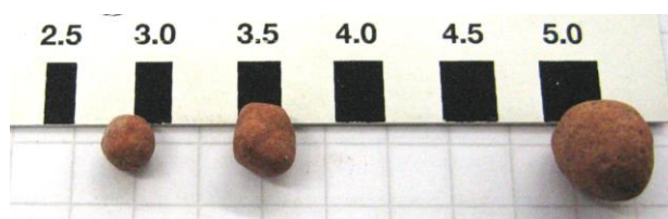
Figure 2.9: LWA of different size (mm) made of expanded clay (Liapor) [Mönnig 2009].
