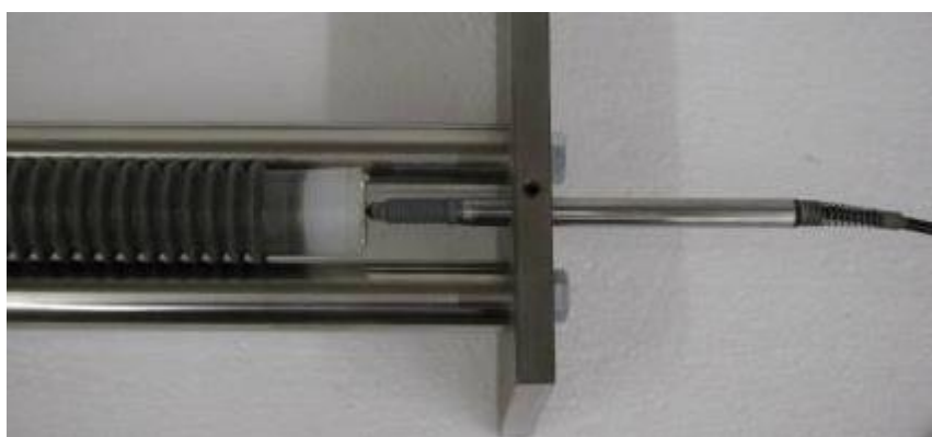
Figure 6.1: Connection detail (free end) of corrugated tube mould embedded horizontally in dilatometer for autogenous deformation measurement.
