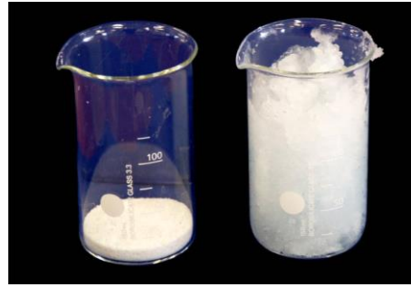
Figure 2.10: SAP particles in dry condition (left) and the same amount of SAP after absorption of tap water [Schwarz 2005] as cited in [Mönnig 2009].
