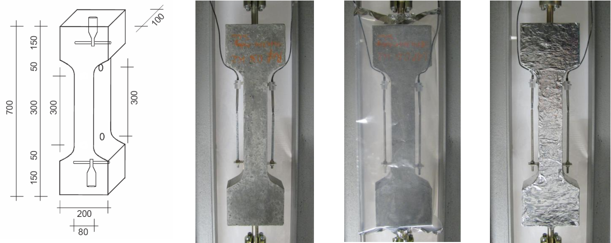
Figure 8.1: Dog-bone shaped specimens: drawing in mm, unsealed test sample, test sample in PE-envelope, test sample sealed by aluminium vapour barrier foil (from left to right).
