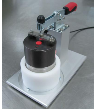
Figure 6.2: Rotronic station equipped with AW-DIO sensor for RH measurement.
