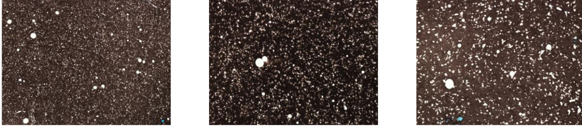
Figure 4.5: Microsections ( 27 \times 20 \text{ mm}^2 ) of hardened cement pastes containing 0.25% SAP A of different size fraction: <63 \mu\text{m} , 63\text{-}125 \mu\text{m} and 125\text{-}250 \mu\text{m} (from left to right).
