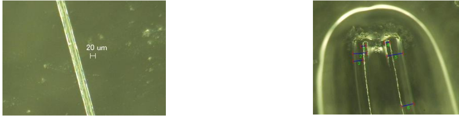
Figure 4.4: Micrograph of polymer fibre SAF in dry condition (left) and after saturation with tap water (right).
