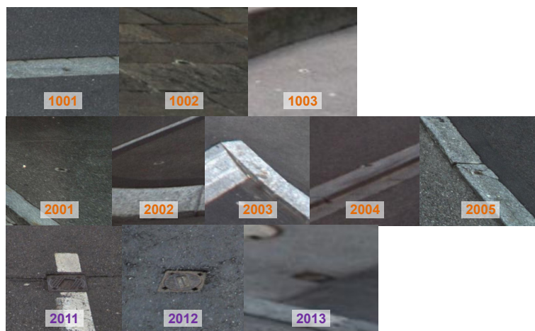
Figure 4.22: Image sections of all 11 3D reference points used for the dataset Zug17. Top row: 3D points in test site I, middle row: visible 3D points in test site II, bottom row: 3D points in manholes in test site II.
