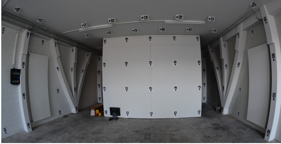
Figure 3.4: Indoor calibration field that is utilized for calibrating IOPs and ROPs (Source: iNovitas).
