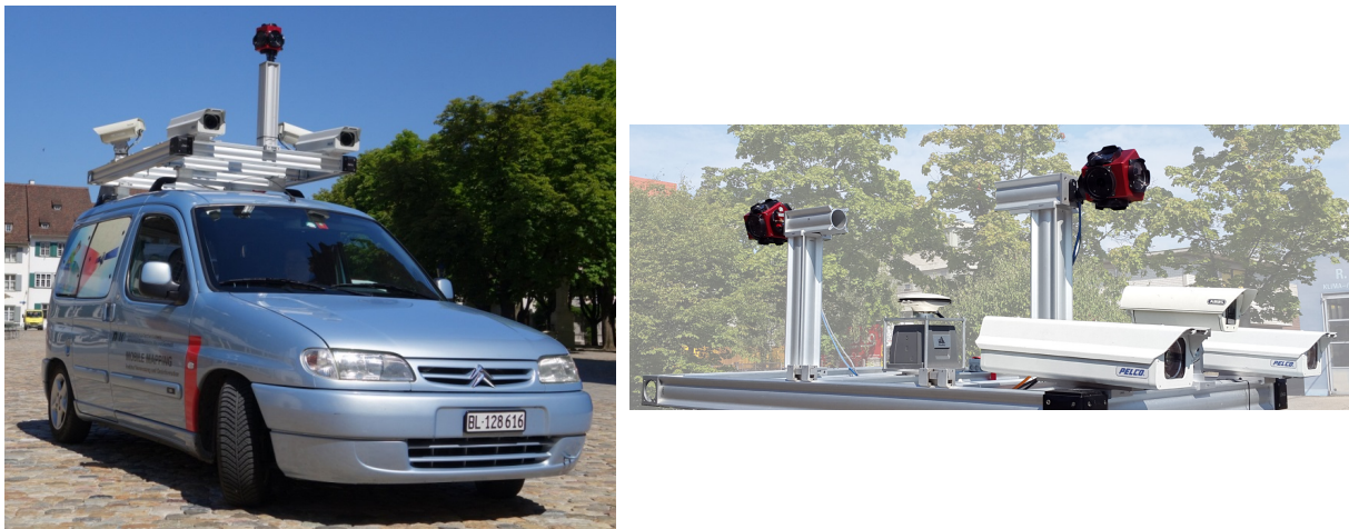
Figure 4.1: Multi-view multi-sensor stereovision IGEO mobile mapping system with sensor configuration for the campaign in July 2014 (left) and for the campaign in August 2015 (right).
