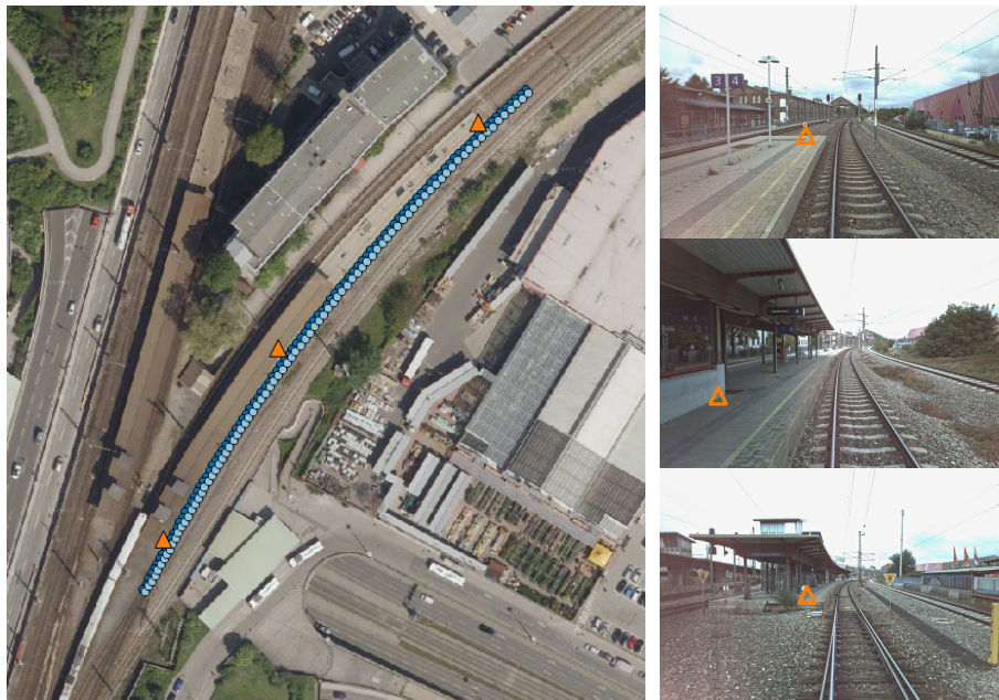
Figure 4.24: Orthophoto of the study area with overlaid blue trajectories and orange 3D check points (left) (Source of orthophoto: Stadt Wien - data.wien.gv.at). Furthermore, there are mobile mapping images from the left camera of the forward pointing stereo system with overlaid orange 3D check points (right).
