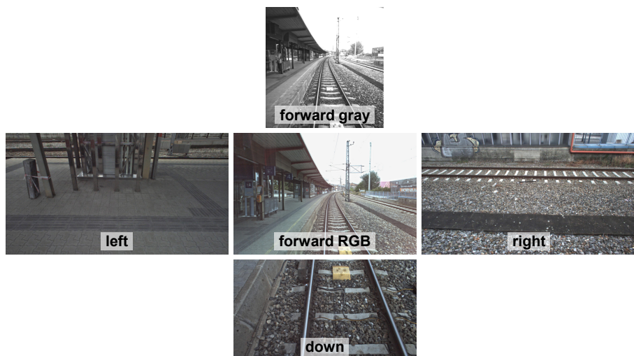
Figure 4.25: Images of left cameras of all stereo systems captured at the same location.
