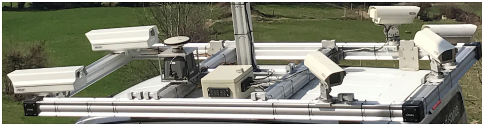
Figure 4.20: Camera configuration that captured the dataset Zug17 (Source: iNovitas).
