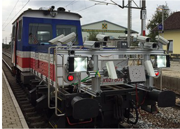
Figure 4.23: Mobile mapping system assembled for a rail campaign in Vienna (Source: iNovitas).
