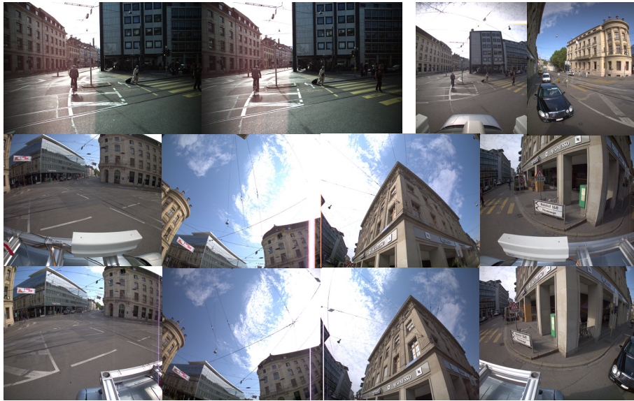
Figure 4.2: Mobile mapping images captured by all cameras at the same location during the campaign in August 2015 (forward stereo [top left], panorama forward and backward [top right], panorama stereo [middle and bottom]).
