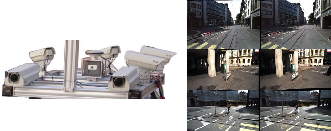
Figure 3.1: Camera configuration (left) and images captured by all cameras at the same location during a mobile mapping campaign in Basel in July 2014 (right: forward stereo [top], back-right stereo [middle], left stereo [bottom]).
