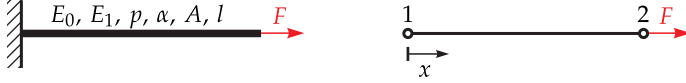
Figure 6.2: Fractional viscoelastic rod (left) described as a two-node one-dimensional finite element (right).
