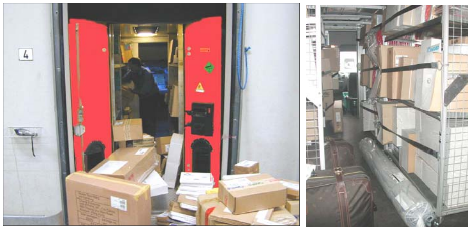
Illustration 2: Vehicle loading: today and by the use of modular racks
