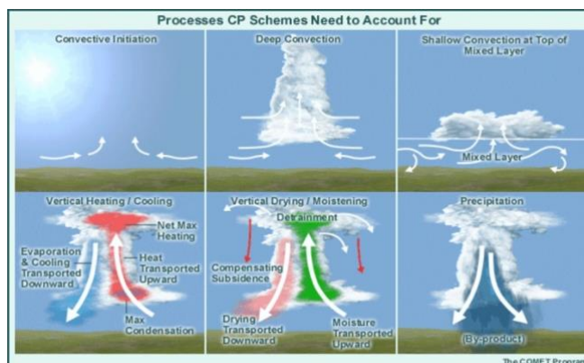
Figure 1: The main processes occurring due to convection. These processes have to be accounted for in convective parameterization schemes. Figure from The COMET Program [14].
