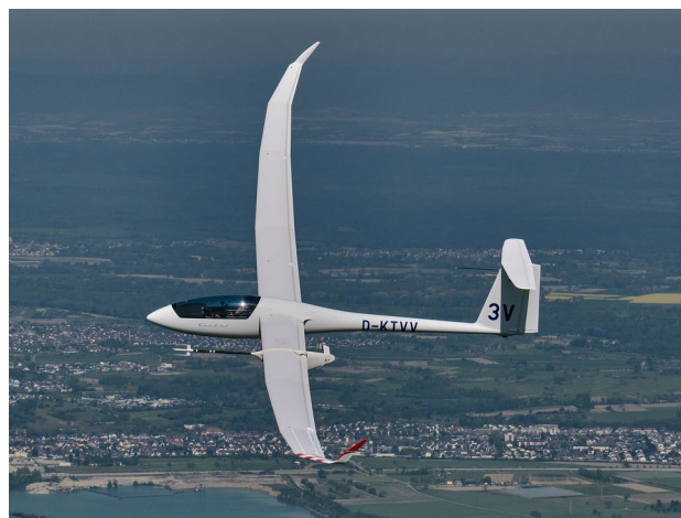
Fig. 4 Test sailplane Ventus 3TS with mounted measurement system on the left wing during a test flight
