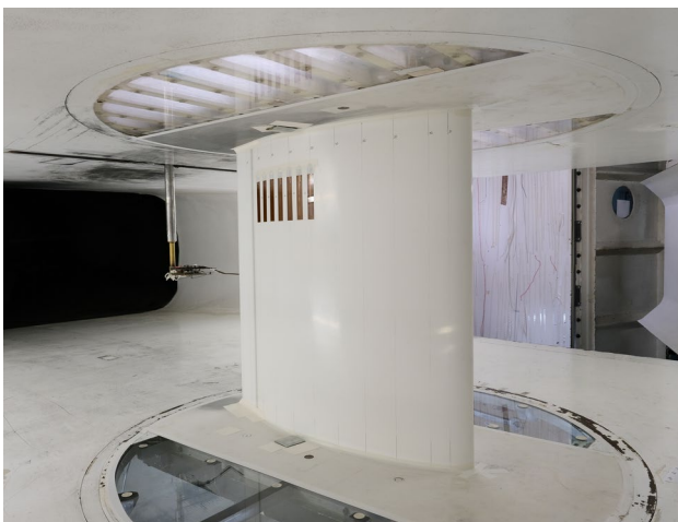
Fig. 5 Test section of the LWT with the WW14k130 airfoil, hot-film sensors (brown stripes) applied in the upper part of the model
