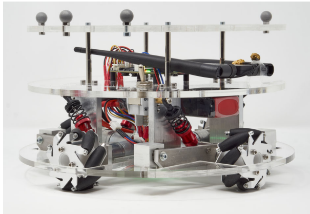
Fig. 2 Omnidirectional mobile robot used as an agent in the robot swarm [1]
