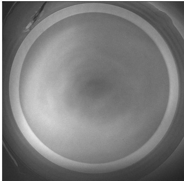
Figure 4.6: TXM cross-section image of the glass fibre used as a substrate for the multilayer zone plate.
