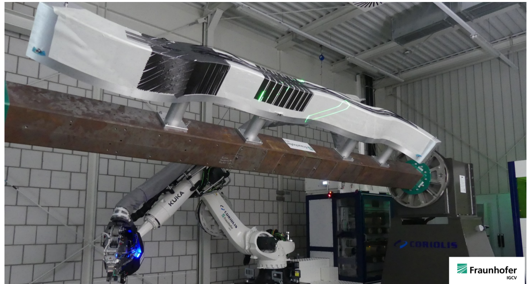
Figure 17. AFP lay-up experiment at Fraunhofer IGCV.
