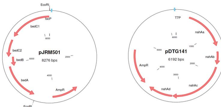
**Figure 4:** The plasmids pJRM501 (left) and pDTG141 (right) encoding the RO genes for BDO and NDO. pJRM501 is based on the pKK223-3 vector containing an ampicillin resistance gene (AmpR) and BDO genes are under the control of the IPTG-inducible *tacP*.<sup>148</sup> pDTG141 is based on the pT7-5 vector harboring an ampicillin resistance gene (AmpR) and NDO genes are under the control of the T7 promoter (T7P).<sup>92</sup>
