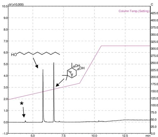
**Figure 8:** GC-FID chromatogram of the CDO M232A-catalyzed biotransformation of (+)- $\alpha$ -pinene **6**. (\*): potential byproduct.
