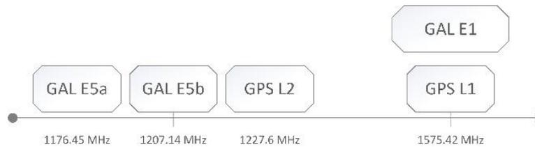
Figure 3-2: GPS L1/L2 and Galileo E1/E5a/E5b frequency bands (Sanz Subirana et al. 2011)
