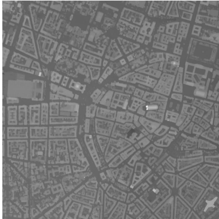
Figure 4.26: The fused DSM generated via our tSGM-based pipeline with WorldView-2 MVS images
