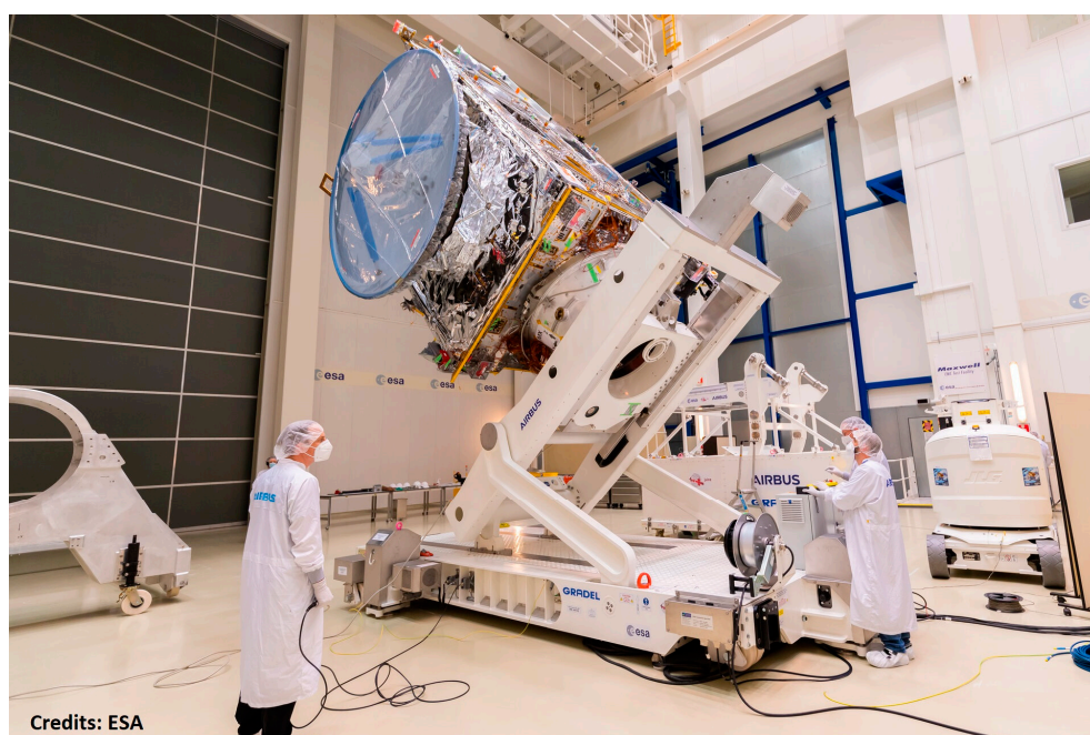
Figure 1. Basic MGSE design [2].
