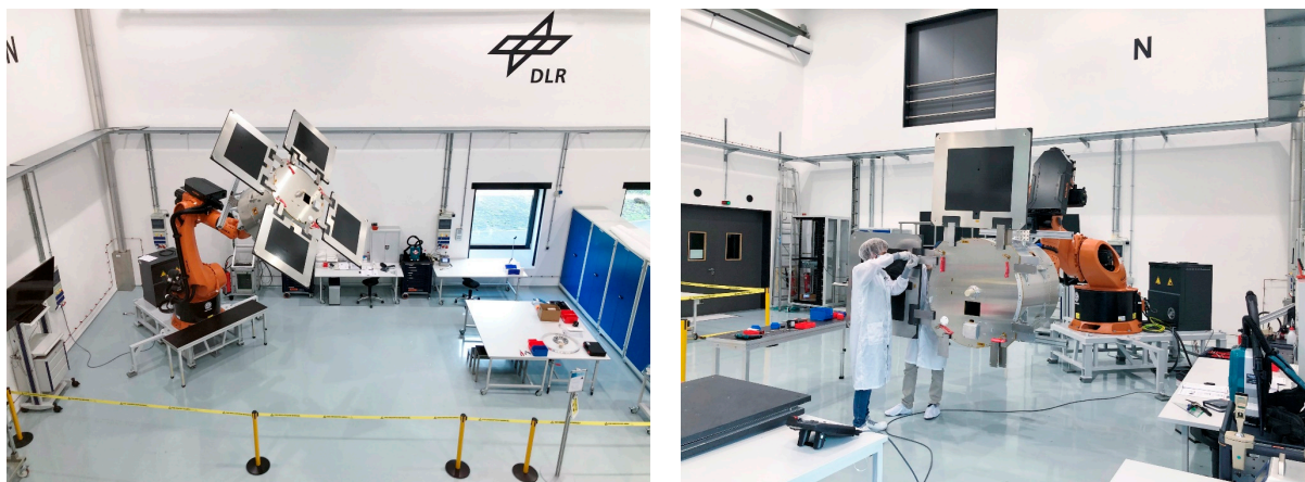
Figure 3. Robotic ground support equipment holding the compact satellite Eu:CROPIS at the DLR integration facility in Bremen ( left ); demonstration of RGSE-assisted integration of solar arrays ( right ).
