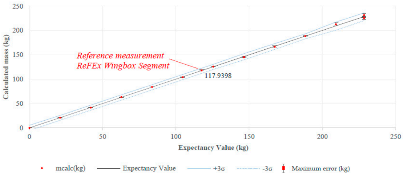
Figure 30. Reference measurement results for the ReFEx Wing box segment.
