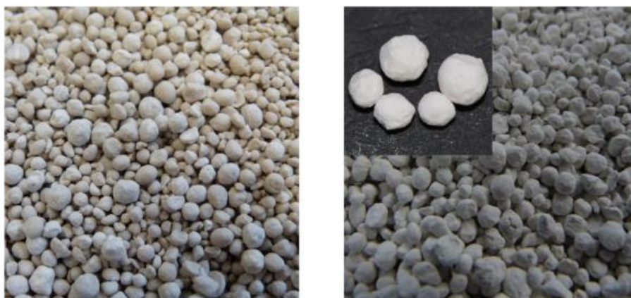
Fig. 9b. State of the sample \text{Al}_2\text{O}_3 before (left) and after (right) the experiment series.
