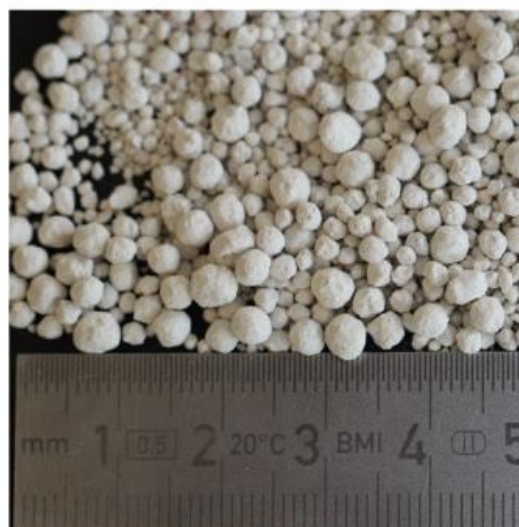
Fig. 3. Reference material – Ca(OH) 2 granules.
