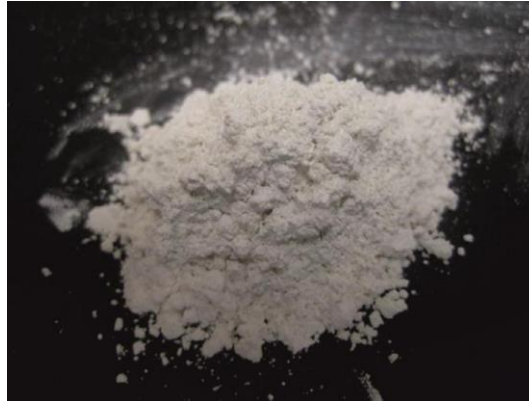
Fig. 4. Left: Calcium hydroxide powder with 0.5 wt% additive after 4 cycles in the lab scale reactor [43]
