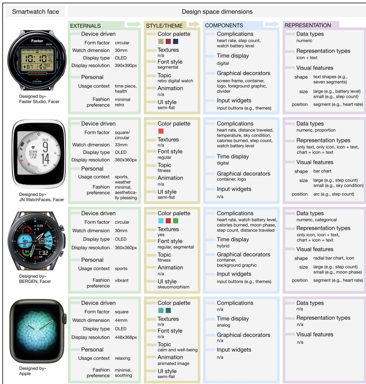
Figure 7. Four examples of smartwatch faces using our design space dimensions to describe them.
