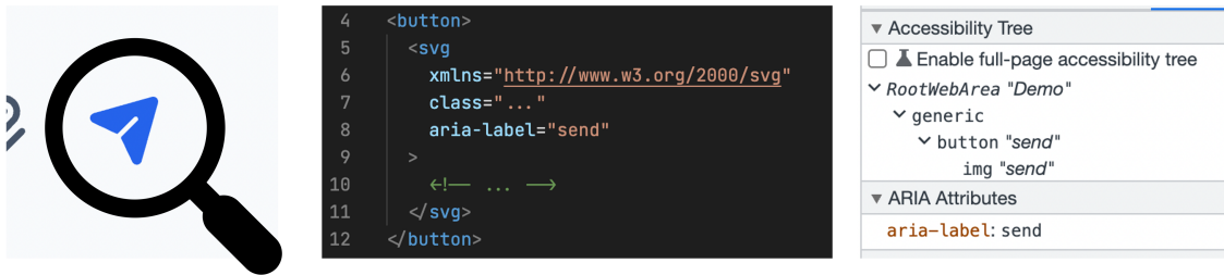
Figure 6.4: Left: Screenshot of an icon of the semantic class “send”; Center: Markup of the icon annotated with an WAI-ARIA attribute by the browser extension; Right: Generated accessibility tree of the icon by the browser
