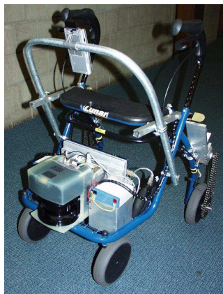
CMU robotically augmented walker [Glover2003, Glover2004]
