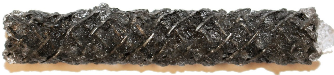
Figure 1: Static mixing element filled with fouling deposits after the polymerization of N-Vinylpyrrolidone in a Fluitec ContiPlant reactor.
