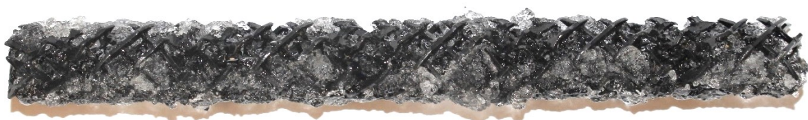
Figure 46: Dismounted DLC-coated mixing element after an operation time of 26 h.
