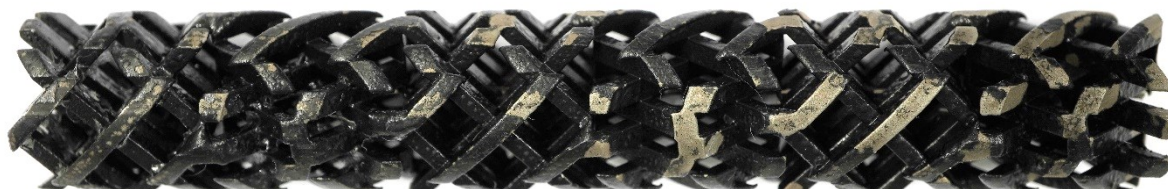
Figure 30: Coated stainless-steel mixer with a teflon coating after multiple studies in a Fluitec ContiPlant reactor.
