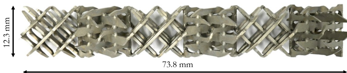
Figure 34: Single static mixing element with the Fluitec CSE-XD6 geometry. Applied from [54].
