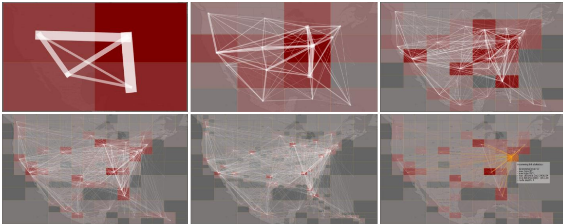
Figure 3.10 — Node-link visualization of the hierarchically aggregated graph. From top left to bottom center: Decreasing levels of aggregation using the computed hierarchy. The thickness of edges encodes the number of movements from cell to cell. Each cell is colored based on incoming or outgoing movements. Statistics can be derived through interactions (bottom right).
