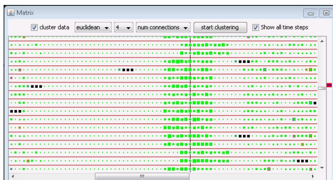
◀ Figure 6.4 — The matrix shows sequences of 192 million computer log events, clustered with k-means . The cluster in the viewport shows machines with high connection counts at a certain timespan and healthy policy status.
