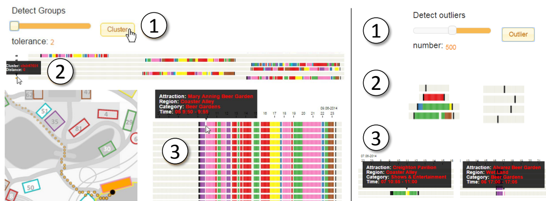
Figure 6.6 — Interactive clustering and outlier detection in attraction visit sequences of amusement park visitors. Left: (1) define the hierarchy cutting level; (2) inspect cluster representatives; (3) inspect cluster members and geographic aspects; Right: (1) define outlier threshold; (2) largest outliers; (3) inspect details.
