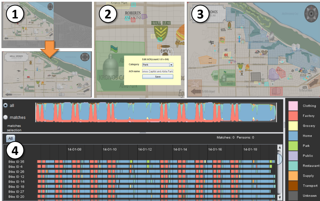
Figure 4.24 — The tourist map is loaded as map overlay and can be aligned to the underlying structure using translation & scaling (1). Subsequently, annotation is used to add areas of interest (2, 3). Accordingly, the linear event sequence visualization (4) reveals frequent behavior such as working, eating, and homecoming.
