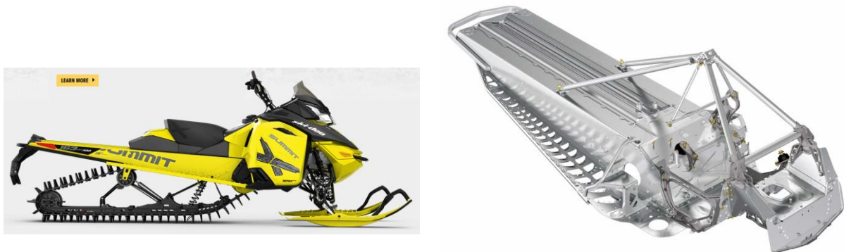
Figure 3: Snow mobile and aluminum chassis with integrated engine chiller, pictures: Bombardier Recreational Products (BRP)
