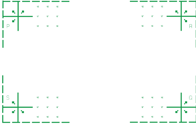
Figure 3.8: The system of four global marks used for exposure layers alignment. Marks are positioned in corners of the exposure field.
