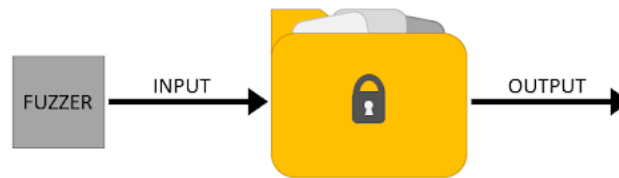
Figure 2.1: An illustration of Blackbox-Fuzzing - the fuzzer has limited access and knowledge to the SUT.
