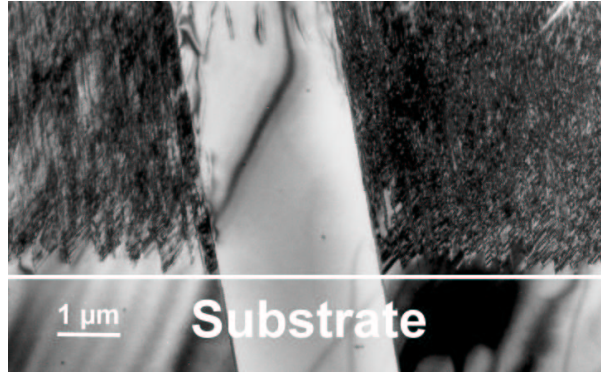
Figure 6.7: Transmission electron micrograph (cross section, bright field image) of an epitaxial thin film on polycrystalline substrate. In the two dark appearing grains nucleation of a high density of structural defects on the substrate surface is observed, while the epitaxial growth in the bright grain in the middle starts defect free at the substrate surface.
