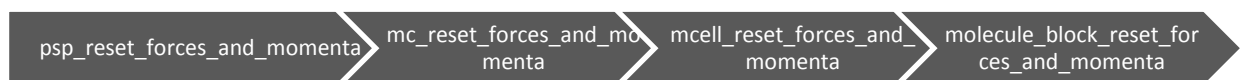
Figure 5.5(c): Sequence of calls for resetting forces of molecules inside phase space
