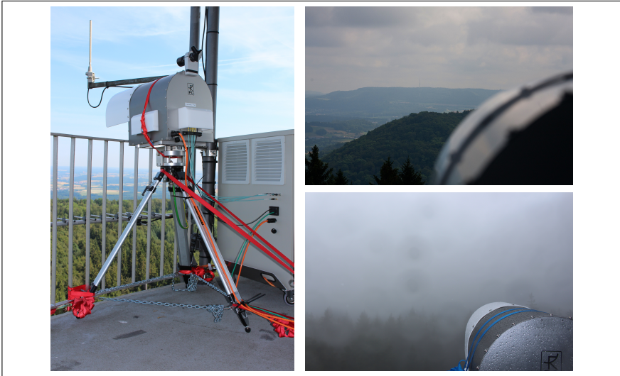
Figure 4.9: Photographs of the 15.7 km transmission experiment with the setup of the transmitter system shown on the left. The photographs on the right show the view from the receiver towards the transmitter site under clear and adverse weather conditions. The Tx's communication tower can be faintly seen in the hills in the background.
